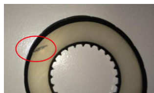
Sample 2: Installation damage
