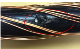
Sample 1: Discontinuity in outer semiconducting layer
