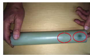
Sample 3: Contaminants introduced during manufacturing
