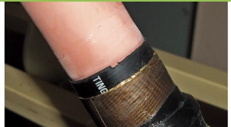
Aged cable defect was pinpointed by a field partial discharge (PD) test matching factory test standards in Table 1 test but not visible with an online test
