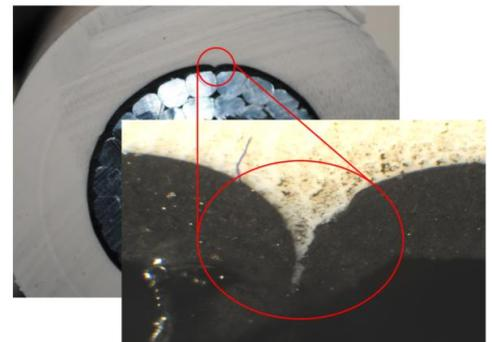
"Fall in" on the conductor shield/insulation interface
