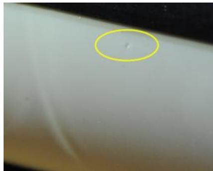
Void on insulation shield/insulation interface
