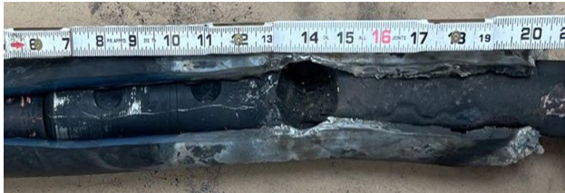
DIMENSION CUTBACK TO CUTBACK = 20 ½" SPECIFICATION - NOT BE GREATER THAN 19 ¾"
