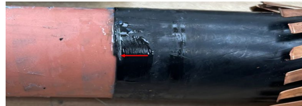
SEMI-CON CUTBACK IS NON-RADIAL
