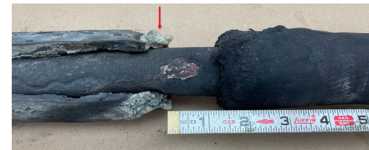
SPLICE BODY NOT OVERLAPPING SEMI-CON
